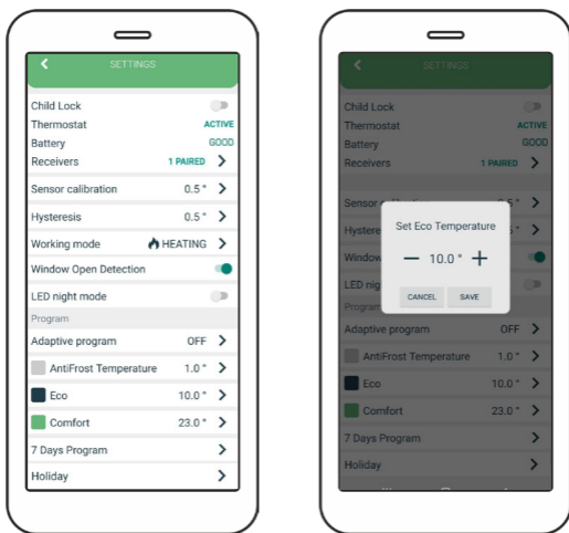
Overview of the screen for setting the economic temperature
