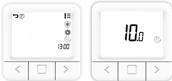
The screen for setting the Eco temperature
